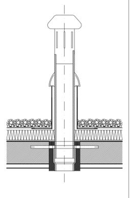
**POZZETTO RACCOLTA ACQUE METEORICHE IN COPERTURA**
